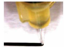
Extrusion printing is used for the controlled deposition of carbon nanotube networks using the biopolymer gellan gum. The biopolymer is an excellent dispersant for carbon nanotubes and thickener for the inks. The actuating and strain gauging ability of printed flexible electrically conducting networks is demonstrated.
