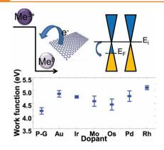
A chemical approach to controlling the work function of graphene is investigated. The work function of graphene increases from 4.2 eV to 5.0, 4.9, 4.8, 4.68, 5.0, and 5.14 eV for the graphene with 20 mm AuCl<sub>3</sub>, IrCl<sub>3</sub>, MoCl<sub>3</sub>, OsCl<sub>3</sub>, PdCl<sub>2</sub>, and RhCl<sub>3</sub>, respectively. Spontaneous charge transfer occurs from graphene to the metal ions, increasing the work function.
