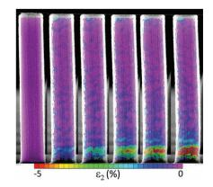
Spatial mapping of deformation fields within CNT array columns is achieved using digital image correlation of in situ scanning electron microscopy (SEM) compression sequences. Strain is highly non-uniform, with buckle formation occurring in localized regions of enhanced strain. A local buckling criterion of 5% principal strain is observed for all columns despite systematic column deformation variation as a function of aspect ratio.
