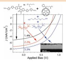
A family of solvent additives is selected based on Hansen solubility parameters and applied to molecular bulk-heterojunction photovoltaic cells. The power conversion efficiency (PCE) and morphology are shown to correlate strongly with the solubility of the donor and acceptor in the solvent additive. By combining solvent additives with complementary effects, the PCE is increased from 1.4% to 3.3%.
