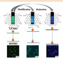
The preparation of controllable fluorescent graphene quantum dots (GQDs) using a new surface chemistry tuning method is reported. The photoluminescence (PL) mechanism is investigated and the competition between both the defect state emission and intrinsic state emission are analyzed in detail. Moreover, the upconversion PL of GQDs is successfully used in multiphoton luminescent biolabeling under near-IR excitation.
